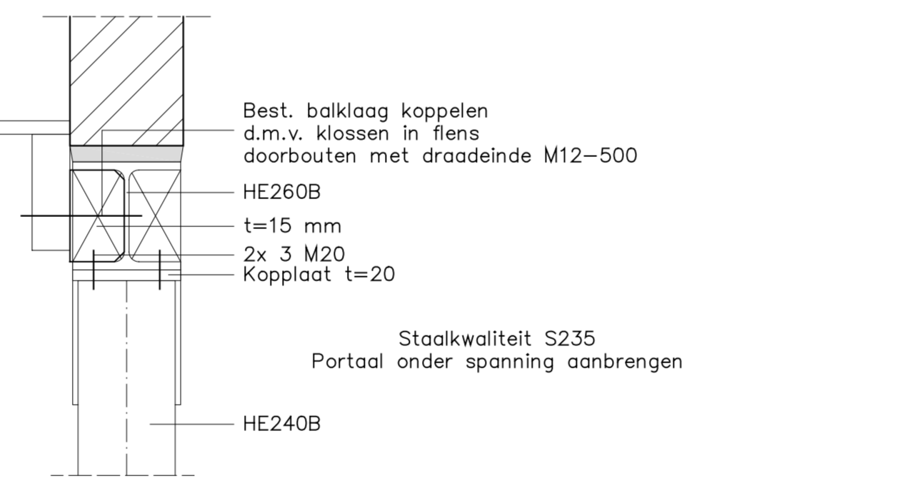
DETAIL C5dws. (bovendetail portaal)
